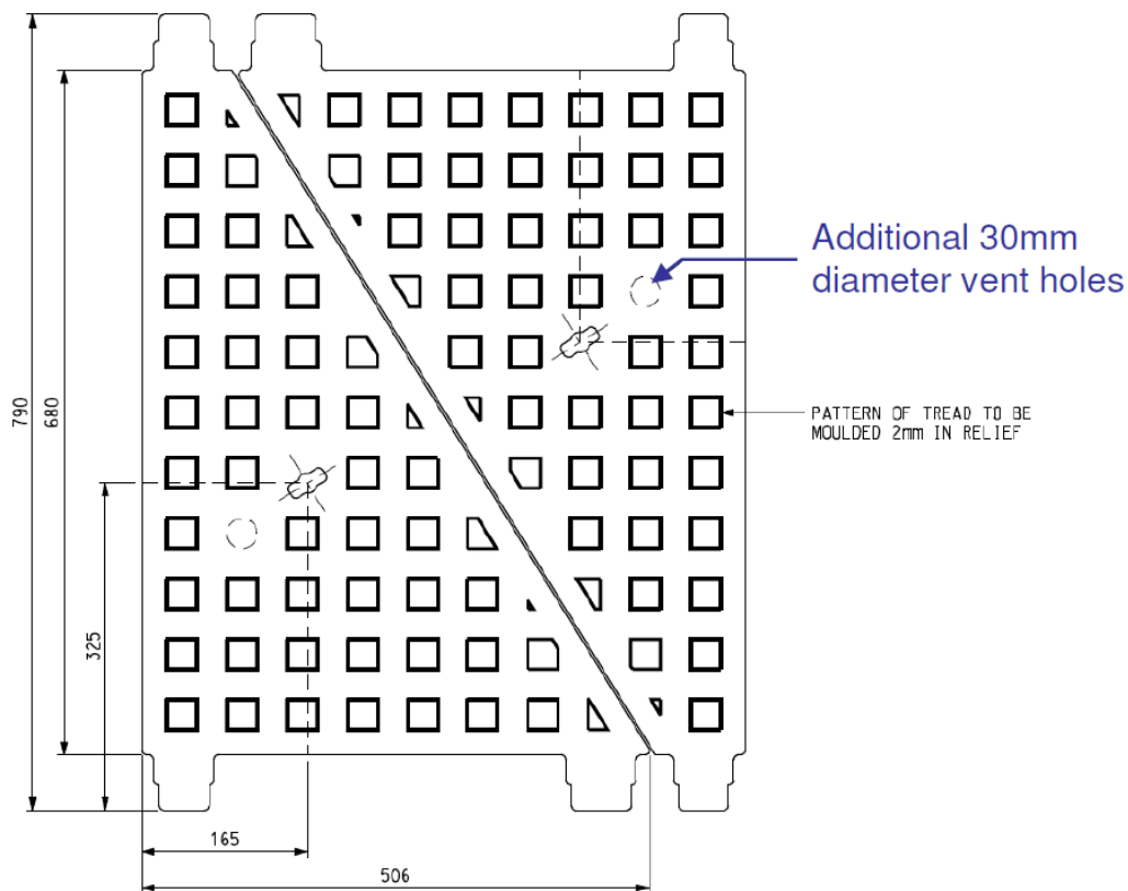
Figure 2: Schematic Layout of Vent Hole in the New Design for Cast Iron Manhole Cover
