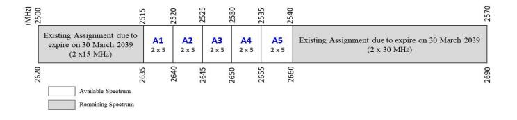
The FDD mode of operation means that the uplink and downlink communications are separated in the frequency domain via different frequencies.
