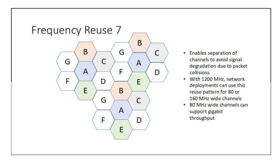
The frequency reuse 7 methodology minimizes packet collisions that degrade throughput by keeping "like" channels separated. With the full 1200 MHz authorized,
